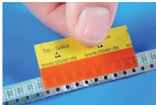
4. apply TOP-Splice to the edge of the Cover Tape and firmly press together
